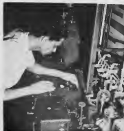
USING INFRARED analyzer, operator Maurice Peterson can rapidly estimate octane rating of alkylate sample.
